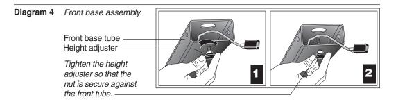
4. Thread the height adjuster to its lowest position. Diagram 4, #1 and #2. Remove the height adjuster from the Hardware kit. Ask an assistant to lift the front base tube while you insert the height adjuster. Turn the height adjuster so that the threads appear inside the base tube. Tighten the nut (with a crescent wrench) when the height adjuster is fully threaded into the front base tube.
